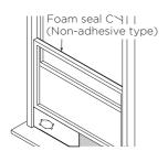
3. Cut the non-adhesive foam seal C strip to match the width of the window. Insert the seal between the glass and the window frame to prevent air and insects from getting into the room.
