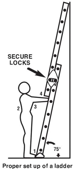
Proper set up of a ladder
