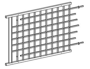
Insert 78" vertical rails (part 9) through cross rails.
