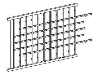
Insert 80" vertical rails (part 8) through cross rails.
