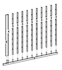
Lay out one right post (part 2). Starting at bottom, insert bottom support rail (part 5), bottom cross rail (part 4) and center cross rails (part 3).
