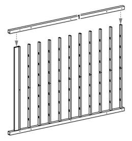
Slide left post (part 1) over corresponding support and cross rails.
