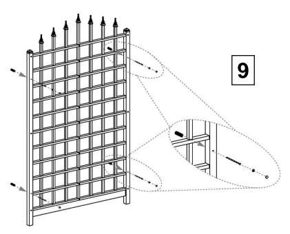
To secure to wall, slide 6" screw through clear screw backer. Insert screw through pre-drilled hole in post. To set trellis away from wall, slide screw through spacer tube. After securing, snap screw cap over screw backer.
