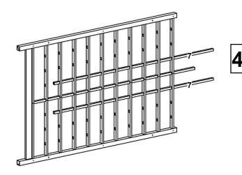
Working outward away from center, insert 82" vertical rails (part 7) through cross rails.
