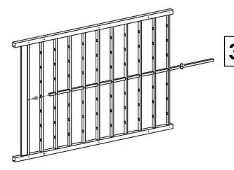
Starting with center hole, insert 84" vertical rail (part 6) through cross rails.
