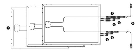
Connect the bare-wire ends of the MC4-to-Bare Wire pair **6** to the charge controller **0**. The positive wire connects to the (+) input and the negative wire connects to the (-) input.
