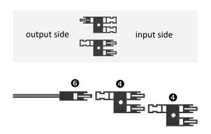
With the other 15-ft MC4-to-Bare-Wire cable **6**, connect one branch connector **4** with the "male" output to the "female" end of the cable. Connect an additional "male" output branch connector **9** to the attached branch connector.
