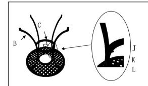
3. Attach part C leg support to part B table legs with four part N studs, four part J flat washers, four part K spring washers, and four part L nuts.
