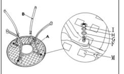
2. Attach part B table legs to part A table top with four part F studs, four part G flat washers, four part H spring washers, and four part I nuts.
