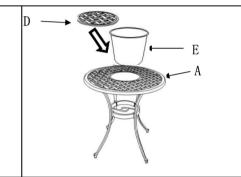
4. Insert part E ice bucket into the middle of part A table top. Place part D cover on top of ice bucket.
