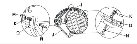
3.Attach part I right arm and part J left arm to part G chair seat with four part N bolts, four part K washers, spring washers, and nuts, and two part M plastic caps.
