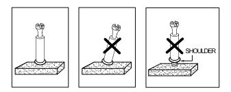
NOTE: Turn the cam-bolt screws until they are tight, the shoulder should be against the surface of the part.
