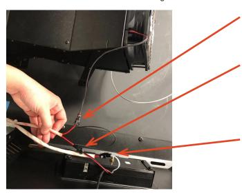
The "black only" wire coming from the fan is connected to one of the "red only" wires coming from the body of the smoker.
