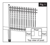
Place the next required post into the dug hole, and slide the post onto the rails of the panel as far as possible.
