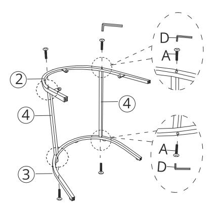
**Step2** First install (5), then tighten all screws on Step 1 and 2 to 100%.
