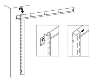
Assemble with hang rail slotted ends to outside. Make sure notches are at the far end of assembled hang rail and space the hang rails on the Top Track 30-3/8" apart measured inside (between) the hang rails. The vertical rails can be mounted to the wall. You can use the provided drywall anchors, the molly bolts or the wood screws if you are mounting to the studs.
