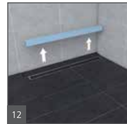
12 Remove the foam block spacer.
