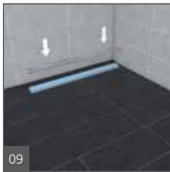
09 Install profile which is now resting on the thinset mortar.
