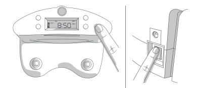
Hold down the ADJUST/SELECT button on the charging station while flipping Bob's power switch ON.
