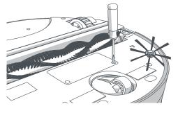
1. Remove the 2 screws on the battery cover using a Phillips head screwdriver.
