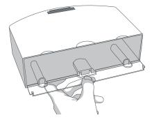
2. Carefully open the plastic gate and dump out the contents of the dustbin.
