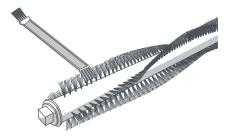
2. Clean the brush and the brush compartment from end to end using Bob's cleaning tool.
