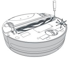
**1**. Remove the screw on the main brush using a flat head screwdriver.
