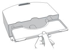
2. Pull out the filter frame from the roof of the dustbin.
