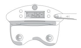
**3.** To select a day of the week, wait until the day stops blinking before pressing the ADJUST/SELECT button to move on. To deselect a day, scroll past it while it is still blinking. Selected days will be lit.
