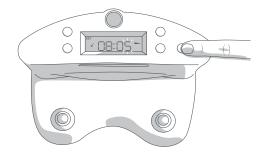
2. Use the ADJUST/SELECT button to adjust your selection. Use the O button to move between minutes, hours, and days of the week.
