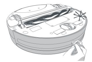
**1**. Wipe the wall and edge sensors using a soft cloth slightly dampened with cold water or alcohol.
