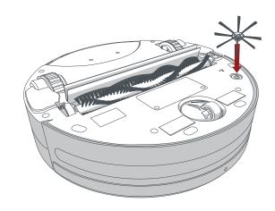
2. Secure Bob's side brush into the socket **1.** Flip Bob over onto a flat surface. Place the side brush over the empty socket on Bob's using the flat head screwdriver and screw. underside.
