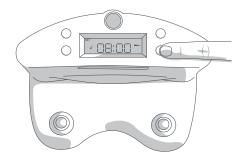
**1.** Press the  $\bigcirc$  button on the station. The first hour digit will start flashing.
