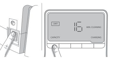
2. While holding down the UV button on Bob's cover, flip Bob's power switch ON.
