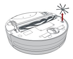
**1**. Remove the screw on the side brush using a flat head screwdriver.
