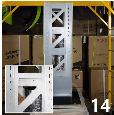
The completed support frames will have 4 sets of screws for each side with the pill-shaped cutouts.
