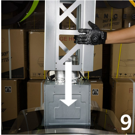
Place the smaller lower support frame and set it into place over the air damper.
