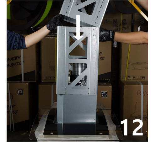
Lift and slip the larger support frame over the smaller one. Adjust it to the ceiling dropdown length desired for your installation.
