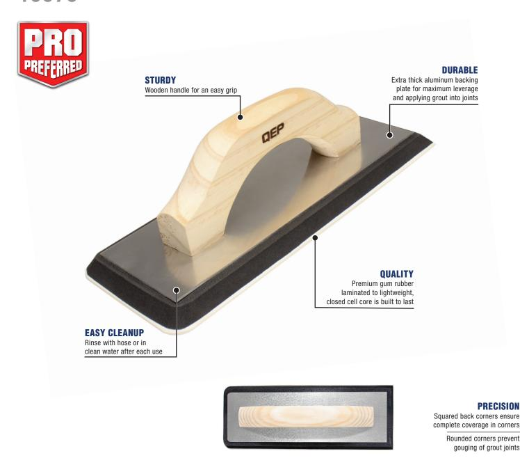
The QEP® Gum Rubber Grout Float features a non-stick gum rubber to ensure grout is applied evenly and smoothly. The 2 rounded corners help prevent gouging at grout joints and 2 square corners help you spread grout in corners and tight areas. The large wood handle allows easy maneuvering and a firm grip. Use for smoothing porcelain and ceramic, textured tile and natural stone. This oversized gum rubber pad is preferred by professional flooring installers.
