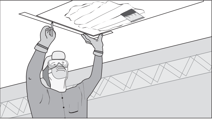
Fig.7. Draw a ractangle the size of the ceiling opening.
