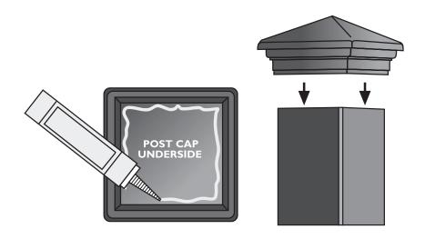
To attach the post cap to the post, apply PVC glue to the underside of the post cap and place firmly on the post.
