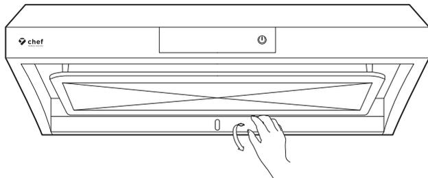
2. Use the clear plastic tray that came with the range hood. Fill the middle section with clean water up to the water level mark.
