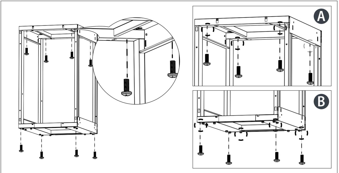
**8** Flip the cabinet frame 180° on a safe and clean surface.
