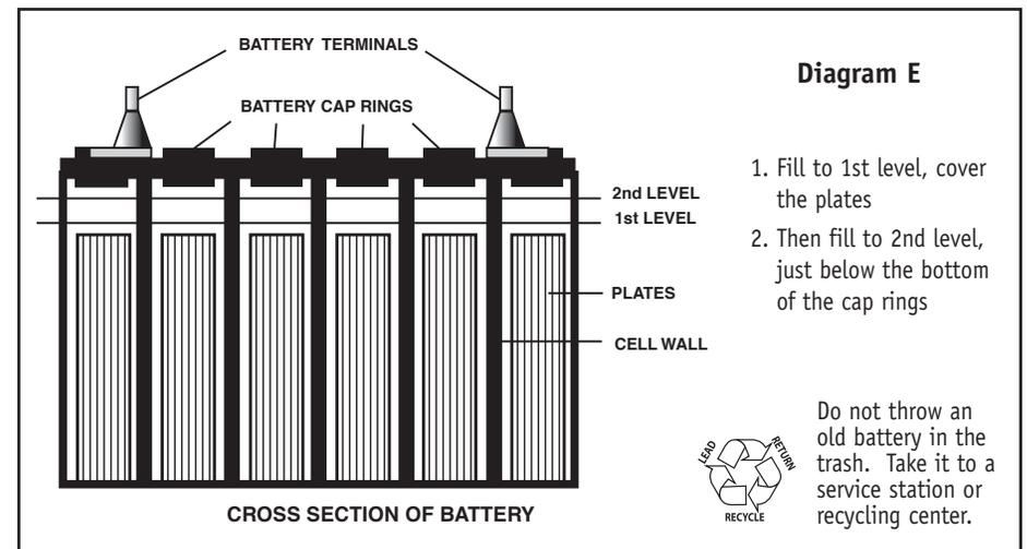
A newly filled battery will sometimes require additional acid after about 20 minutes. Re-examine the fill level, and add additional acid if necessary. The battery acid may bubble at this time and give off a sulfur-like smell, but this is normal. You may top off each cell with a little distilled water, if needed. After the battery has been filled, screw the six (6) caps securely on the top of the battery.
