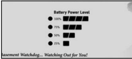
power, or simply by aging, the gauge will indicate the percent of charge remaining in the battery. Should the level drop below 25%, the "Battery problem" indicator will light up and the alarm will sound.
