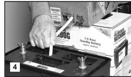
**the battery plates, and then go back and top off each cell equally. It is important to have all the cells filled equally or the battery will not operate properly.** The acid should reach a level about  $\frac{1}{4}$ " below the cap ring as shown in the diagram at right. DO NOT OVERFILL THE BATTERY. (Diagram E)
