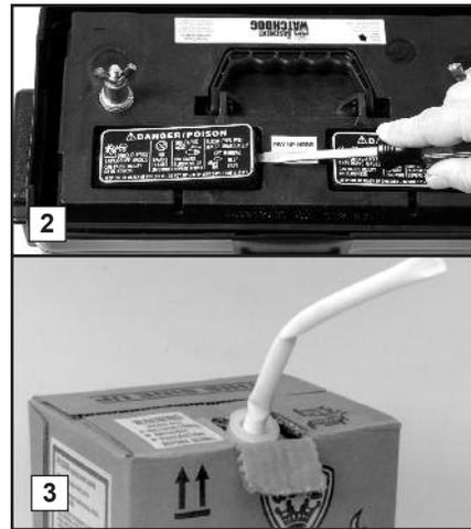
on the right. Place the screwdriver in the middle of the cap on the top of the battery. DO NOT lift the cap by prying it up from the groove on the back of the battery cap. It may damage the vent.
