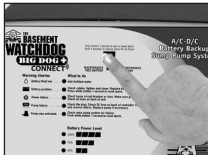
problems. In addition, an alarm sounds to alert you to the problem. In some cases the lights and alarm will go off automatically when the problem has been solved. In others, the BLUE button must be pushed to silence the alarm. Refer to the table below for a quick review of the features and their corresponding alarm status.
