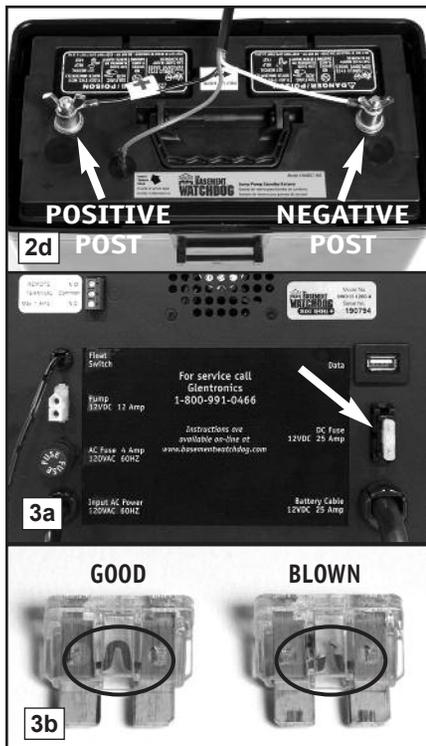
3. (a) Check the DC fuse by pulling it out of the fuse holder. (b) If the wire within the fuse is burned and broken, replace the fuse with a 25 amp DC safety fuse. If the fuse blows again, unplug the computer control unit from the wall and disconnect the battery cables from the battery. Then call Glentronics technical support for instructions at 800-991-0466, option #3. You may need to replace the pump.
