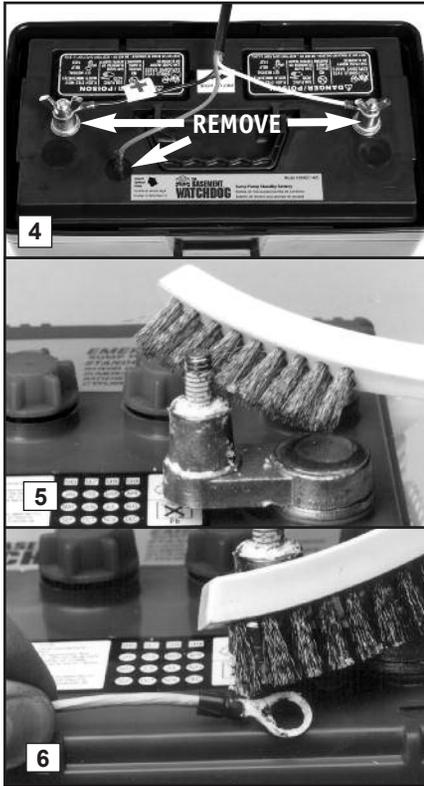
4. Remove the fluid sensor from the top of the battery. Unscrew the wing nuts and remove the battery cables.
