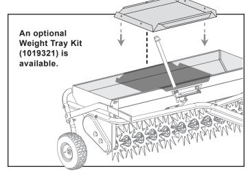
For tougher ground conditions (or to aerate without spreading), an optional weight tray can be added to the Aerator.
