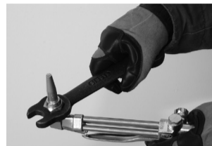
Figure 7. Installing Cutting Tip
