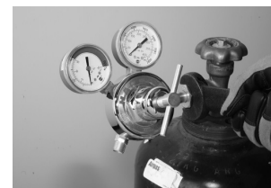
Figure 3. Attaching Fuel Gas Regulator
