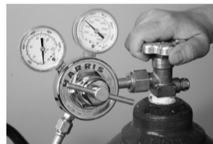
Figure 9. Opening Fuel Gas Cylinder Valve
