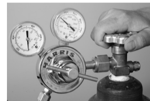
Figure 10. Opening Oxygen valve
