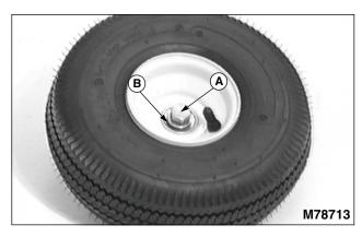
1. Install 1/2 x 3-3/4 in. hex bolt (A) and 1/2 in. flat washer (B) on valve stem side of wheel hub.
