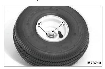
1. Install  $1/2 \times 3-3/4$  in. hex bolt (A) and 1/2 in. flat washer (B) on valve stem side of wheel hub.
