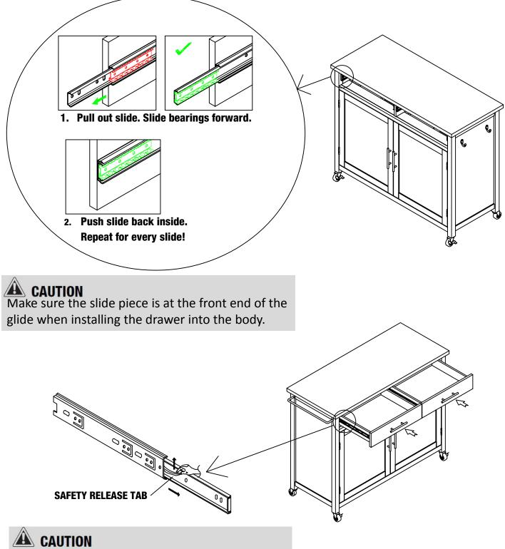
When removing the drawer, tip-up the safety release tab to remove the drawer from the body.
