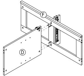
□ **d)** Tighten bolt (GG) with lock (HH) in the pre-drilled holes.
