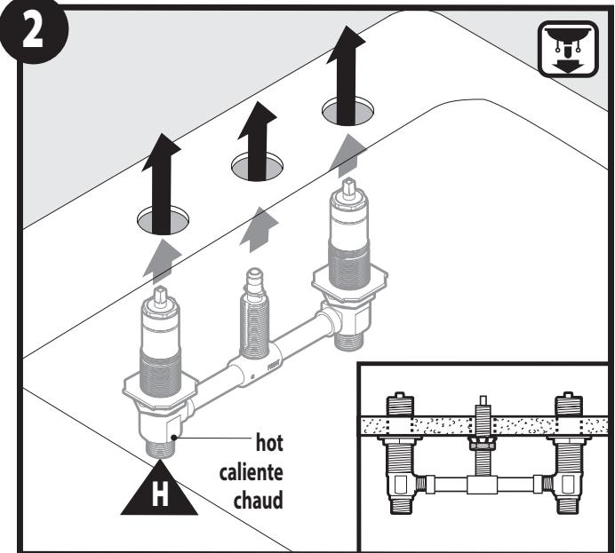
From below sink deck, insert Valve Body (H) up through sink openings. (Note: Hold Valve Body (H) in place for next step instructions.)
