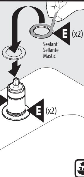
Apply sealant to one side of each Upper Mounting Washers (E). Turn over and install over each portion of Valve Body (H) till seated on sink.
