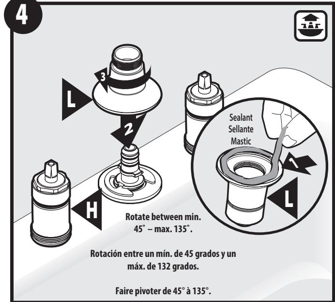
1.) While holding Valve Body (H) in place, apply sealant to underside of Spout Base (L).
