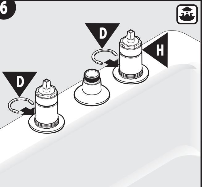
Insert Valve Body Clips (D), one onto each groove of Valve Body (H). Push till clips are secured onto valve.
