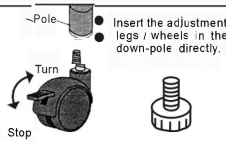
Insert the adjustment legs / wheels in the down-pole directly.
