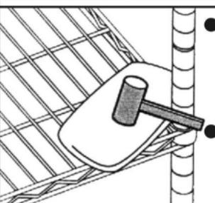
Then, put the mesh flake on the places of pipe nips.
