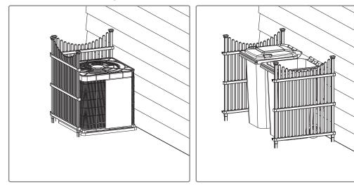
\* Screens are designed to be installed at a right angle for optimal stability. If installing in a straight line or independently from each other, it is recommended to secure the posts into the ground with a bit of gravel or quick drying cement to ensure your screens are not easily knocked over.
