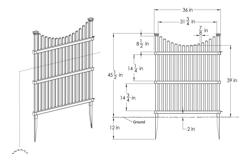
If necessary, this enclosure can be trimmed down vertically to fit your custom space. Use a fine toothed circular or hack saw. Rails will need to be re-spaced and configured accordingly.
