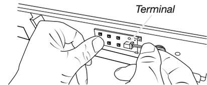
4. Replace a new LED, press it back between two hooks and plug in the terminal.
