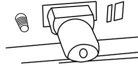
5. Reattach the second top vent cover with the screw removed in step 1.
