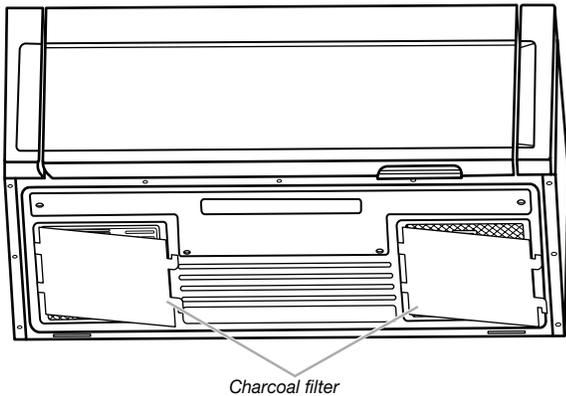
3. Replace a new charcoal filter and reattach it back to the bottom plate, and make sure both left and right sides insert into the bottom plate slots.
