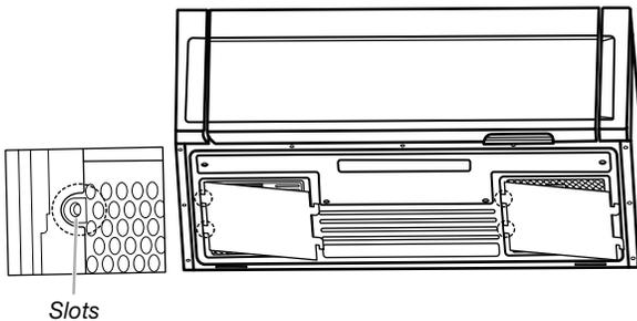
4. Put the grease filter back to the bottom plate.
