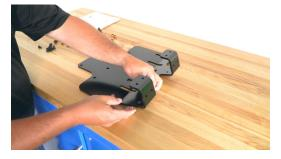
b. Remove the hitch bracket (1/2" wrench required)
