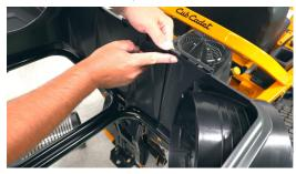
c. Align the cover tabs and use the mounting pin to secure (use a screwdriver to ease the pin into place)
