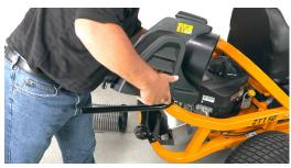
b. Snap plastic top cover support in place (make sure the tab is locked in place)
