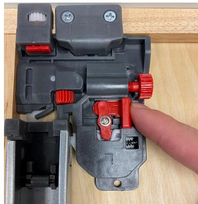
2 Reach underneath drawer box at front and locate runner releases on each side of drawer box.
