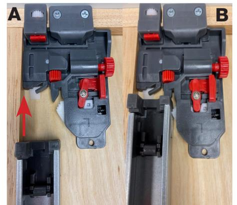
6 To lock drawer box back in place, set the drawer on the runners and fully close until you hear the 'click' of the runners locking into the release tabs. Open and close repeatedly to align runners and ensure lock.
