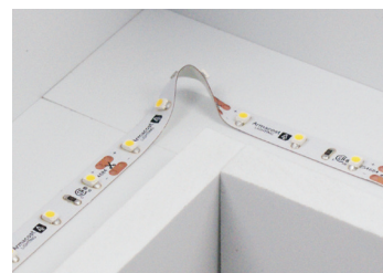
Use loop bend technique for coves and above cabinet installations
