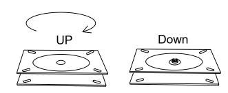
Rotate the top half of component 2 by 45°.
