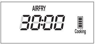
**NOTE:** ■ It can be programmed for four different temperatures. They are: 425°F(default) → 350°F → 375°F → 400°F.
