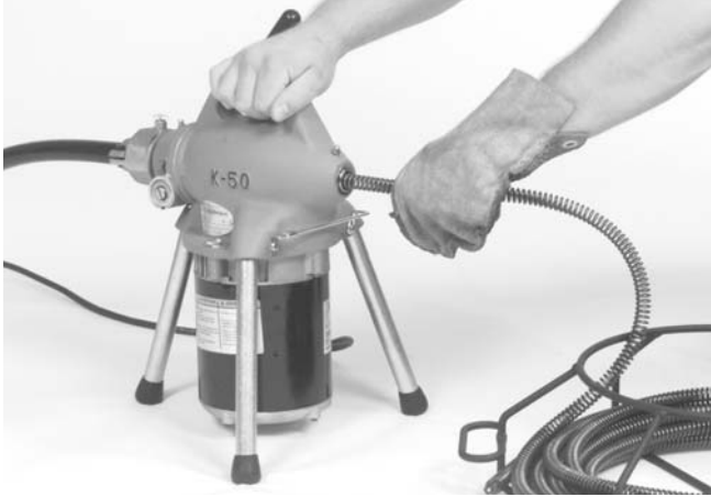
Figure 3 – Inserting Cable Into Front Of Machine
