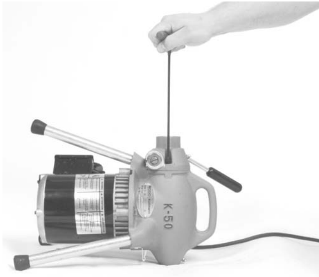
Figure 10 – Remove Socket Head Cap Screws
