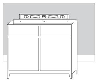
4. Attach the vanity to the wall by screwing through the back of the vanity cabinet. Use the marked stud locations as a guideline. Proceed to Step 2 for attach ing your counter top.
