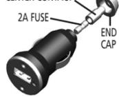
1. Unscrew the end cap counterclockwise and remove.
