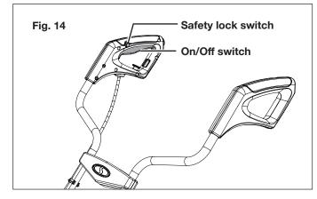
3. To switch OFF, release the ON/OFF switch (Fig. 14).
