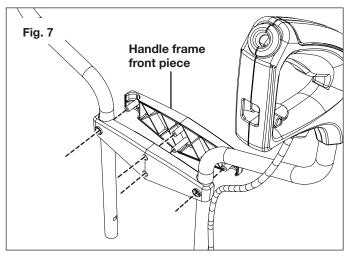
**4.** Join the assembly with the original 4 screws, as shown (Fig. 8).
