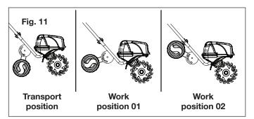
2. To adjust the wheel position, push the wheel adjustment knob while moving it to the slot for desired position; let go of the knob and make sure it locks into position (Fig. 12).
