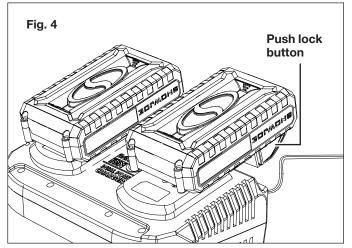
**CAUTION!** FIRE HAZARD. When remove the batteries from the charger, be sure to unplug the charger from the outlet first, then remove the batteries from the charger.
