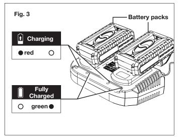
**4.** When the charger lights turn green, the batteries are fully charged (Fig. 3).
