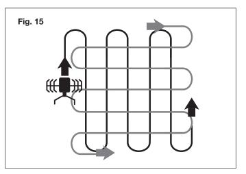
Pay special attention when changing direction. Apply light pressure to the handle in order to lift the blades and facilitate the turn. Turn the product around using the wheels as a guide. Gradually release pressure on the handle and move the blades back to the ground.
