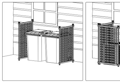
\* Screens are designed to be installed at a right angle for optimal stability. If installing in a straight line or independently from each other, it is recommended to secure the posts into the ground with a bit of gravel or quick drying cement to ensure your screens are not easily knocked over.
