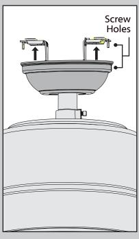
Lift the canopy place so that the screw holes are aligned.
