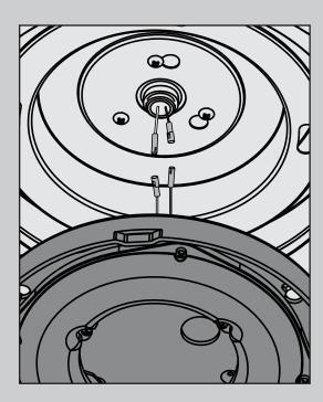
Connect the white wire from the fan to the white wire from the light kit, then connect the black wire from the fan to the black wire from the light kit.
