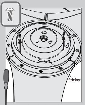
Locate the red sticker on the upper switch housing. Screw two switch housing screws from the ≡ hardware bag halfway into the other two screw holes in the upper switch housing.
