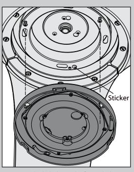
Raise the light kit to the fan with the sticker on the light kit aligned with the sticker on the upper switch housing. Wrap the keyhole slots around the screws and twist the lower light kit clockwise.
