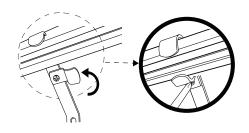
Tighten all set screws on the top of each bracket.
