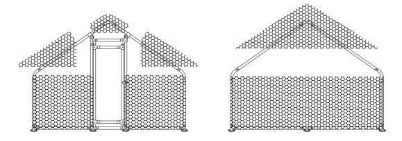
Measure the door size Pre-cut the wire mesh for covering
