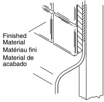
**15** Apply 100% silicone sealant around the bath along the finished walls and deck.
