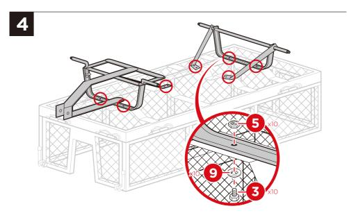
Attach the completed item from step 1 to part A bottom frame using six part 3 bolts, six part 5 nuts, and six part 9 washers.
