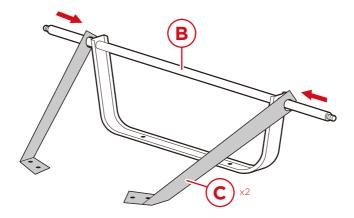
Attach part C rear struts to both ends of part B rear axle frame.
