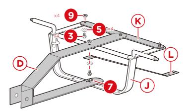
Use a part 3 bolt, part 5 nut, and part 9 flat washer to attach part D yoke, part J front axle, and part L front axle brace together.
