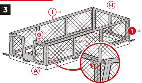
Attach part G front panel, part I side panels, and part H rear panel to part A bottom frame using two part 1 B pins for each panel.
