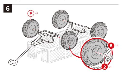
Insert four part F wheels into part J front axle and part B rear axle frame using a part 2 washer and part 6 nut for each wheel. Use the air pump to inflate the wheels to a maximum of 25 PSI.
