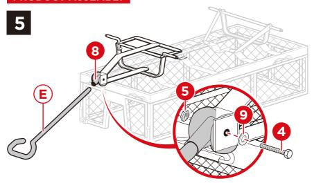
Attach part 8 handle coupler and part E handle to part D yoke using a part 4 bolt, part 5 nut, and part 9 washer.
