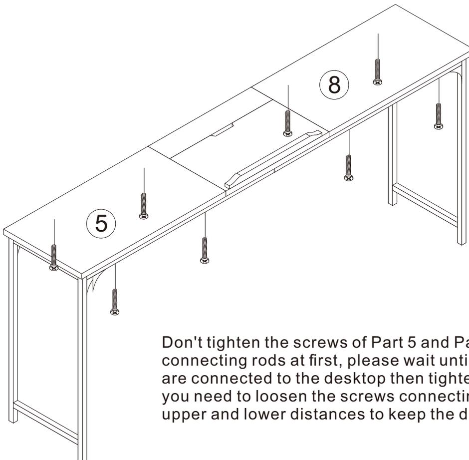
Don't tighten the screws of Part 5 and Part 8 and the bottom connecting rods at first, please wait until Part 9 and Part 10 are connected to the desktop then tighten them. If Part 7 is not flat, you need to loosen the screws connecting Part 4 to fine-tune the upper and lower distances to keep the desktop flat.
