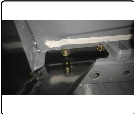
5. Torque all 7/16" hardware to 59 ft-lbs. Re-attach muffler brackets removed in Step 1. Torque all M8 muffler bracket hardware to 23 ft-lbs.
