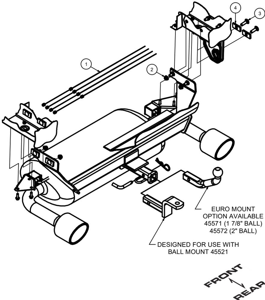
1. Lower exhaust by removing (6) bolts from the muffler brackets, retain bolts for reinstallation.
