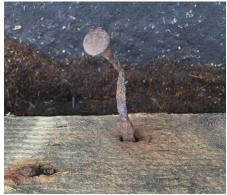
The effect of corrosion on HDG spikes.
