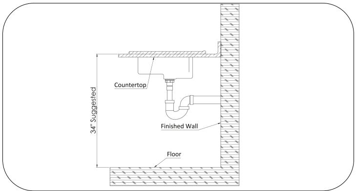
2 Place the vessel sink on the mounting ring or counter top as shown.
