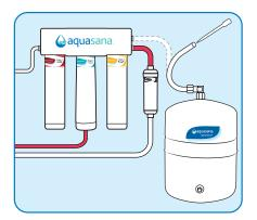
6 Sanitation will be completed during the following pressure test and purge. Important: Bleach must be completely removed from system before drinking water. See Purge instructions below.
