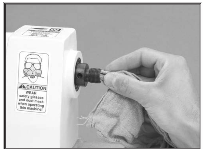
Figure 32. Cleaning spindle tapers.
