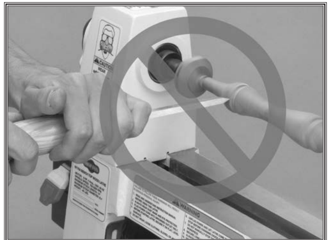
Figure 6. DO NOT cut without using tool rest.
