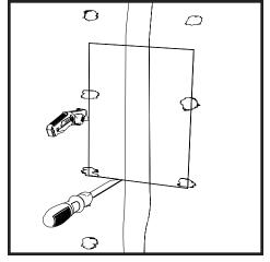
2. Measure the distance between vertical studs. (Please note that the distance between the center lines of 2 adjacent studs generally is 16 inches and the niche is designed for that condition.)
