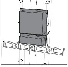
b. Cut out the wall board along the traced lines between the two studs using a drywall saw and utility knife.
