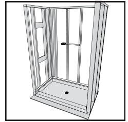
If the distance is greater than 16 inches, attach vertical framing to one or both of the vertical studs to accommodate the size of the niche.
