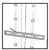
a. Place the niche between the two marked studs with the flange walls flush against the wall and trace the outline of the niche on the wall. Be sure the top and bottom lines are level.
