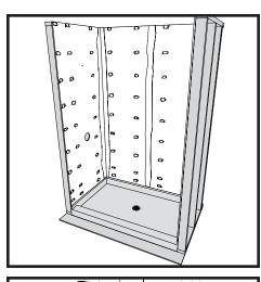
1. If framing Redi Niche into an existing finished wall (if new construction, skip to Step 2), first locate and mark the center of adjacent framing studs using a stud finder or by tapping the wall. Draw a level line between the two wall studs.
