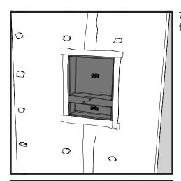
7. Then apply a liquid applied waterproofing membrane to all four niche flanges and covering at least 1 inch of the adjacent tile backer board
