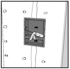
6. Neatly apply 100% waterproofing silicone to cover each screw head and to fill the gap between the niche flange and the adjacent shower board.
