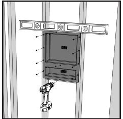
4. Level and mechanically fasten the Redi Niche using one framing screw in each pre-drilled.
