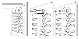
**3** The meat probe icon flashes in the display if the meat probe is properly connected.
